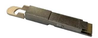
Luxshare-TECH 200Gbps S-QSFP-DD optical transceiver is designed for 200Gbps Ethernet links with short-reach communication. The link distance up to 70m and 100m over OM3 and OM4 respectively. It integrates eight data lanes in each direction with each lane operating at 25.78125Gbps and 10.3125 Gbps. This transceiver also can be used for high density 200G/80G Ethernet applications. They are compliant to IEEE802.3bm 100GBASE-SR4 and breakout 4x25 GBASE-SR and QSFP-DD MSA.
